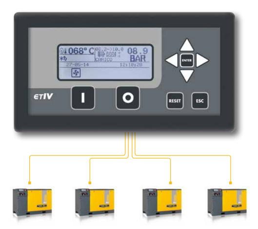
**Master/slave function**: it is possible to connect up to 4 compressors for managing the workload in such a way to equalize the hours of each compressor in a network to ease servicing. The system pressure can be dynamically programmed to various set pressures according to usage.
